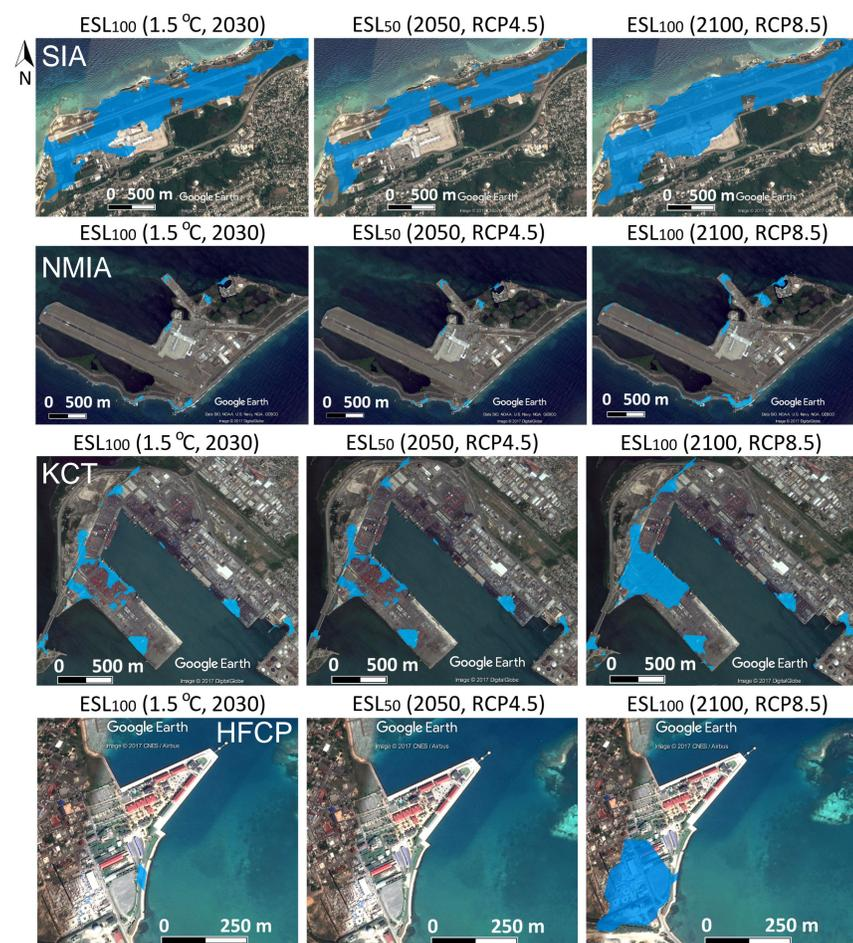
In **Jamaica**, even under the 1.5 °C SWL, the 100-year event will cause considerable flooding of the **SIA** runway. **NMIA** is less prone to coastal inundation. Under the 1.5 °C SWL, some areas of the **KCT** seaport are projected to be flooded under the 100-year event, whereas by 2100 extensive areas will be affected. The **HFCP** cruise port will be very moderately affected until the 2080s.
