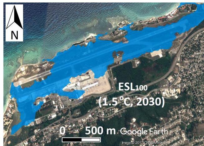
Figure 4. Example inundation modeling from LISCoAsT
