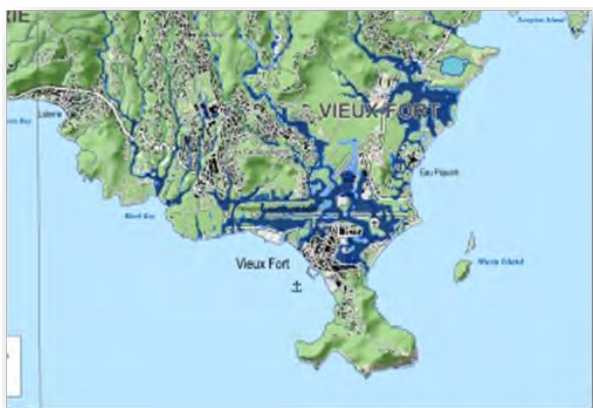
Figure 5-1 Extent of flash Flooding at Hewanorra Airport on 24 December 2013 – Rainfall event of 1:5. (Source: GoSL and World Bank, 2014)
