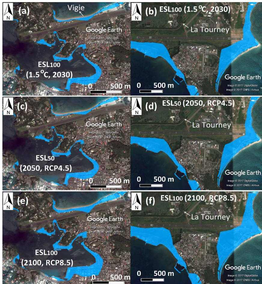
Figure 3: Coastal flooding – Saint Lucia Inundation maps of (a, c, e) GICIA and CSP and (b, d, f) HIA and VFSP under ESL100 (1.5 °C, 2030), ESL50 (2050, RCP4.5) and ESL100 (2100, RCP8.5)
